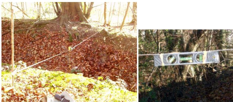
Figure 30. Arrangement for measuring bank and ditch profiles. © DG.
