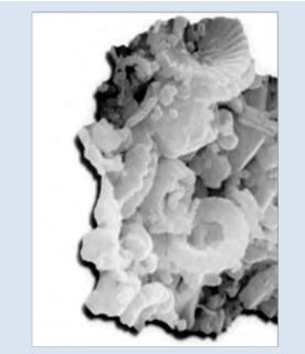
A high resolution image of the tiny chalk particles and the spaces between them. A chalk well can yield more than 10 million litres of water per day, sufficient to provide the needs of about 70,000 people at 150 litres per person per day.
