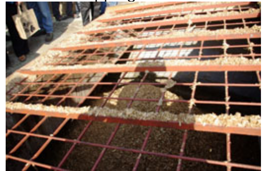
Allows the delivery to drop into the centre of the bunker, keeping the unused space to the minimum
